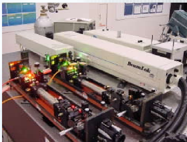
Figure 7. CLA's modelocked laser system provides a versatile multiple-wavelength excitation source with continuous wave, or femtosecond or pico-second pulse durations
