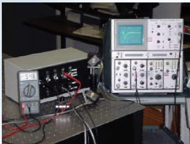
Figure 6. CLA-built control electronics and single-photon avalanche diodes
