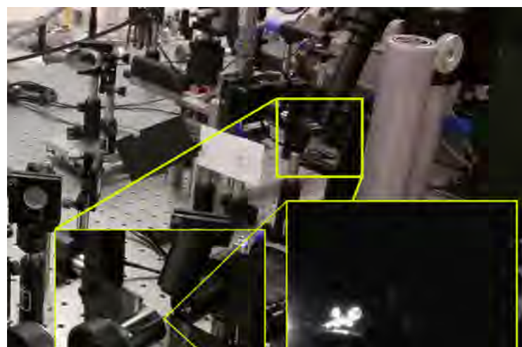
Experiment for time-gated imaging of femtosecond laser nanofabrication. The lower right inset shows nanoparticles ejected from the surface during the formation of nanoholes in a fused silica substrate.
