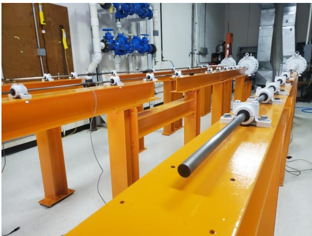
Fig. 1 - Three Split-Hopkinson Pressure Bar Systems for the Measurement of the Dynamic Stress-Strain Response of Materials in Tension, Compression, or Shear Mode. Note: The three systems are currently being refurbished and updated with new instrumentation.
