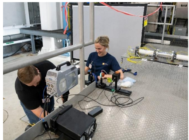
Fig. 2 - Dr. Phil Kreth and Haley Goldston install UTSI's retroreflective shadowgraph system in AEDC's SL-2, a sea level turbine engine test cell at Arnold Air Force Base. U.S. Air Force photo by Jill Pickett.
