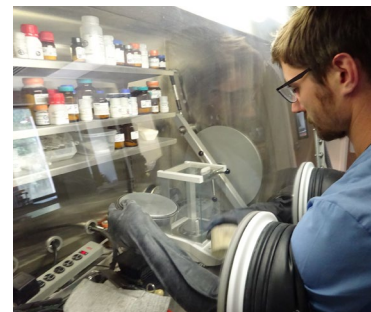
Figure 2. A student prepares a glass sample within an argon atmosphere glovebox.
