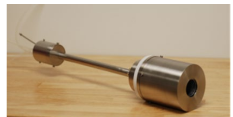
Figure 2. Ion source used in the ion depaint process.
